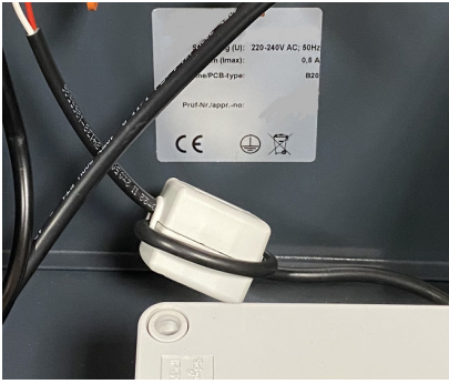
Setting of the air probe T1
